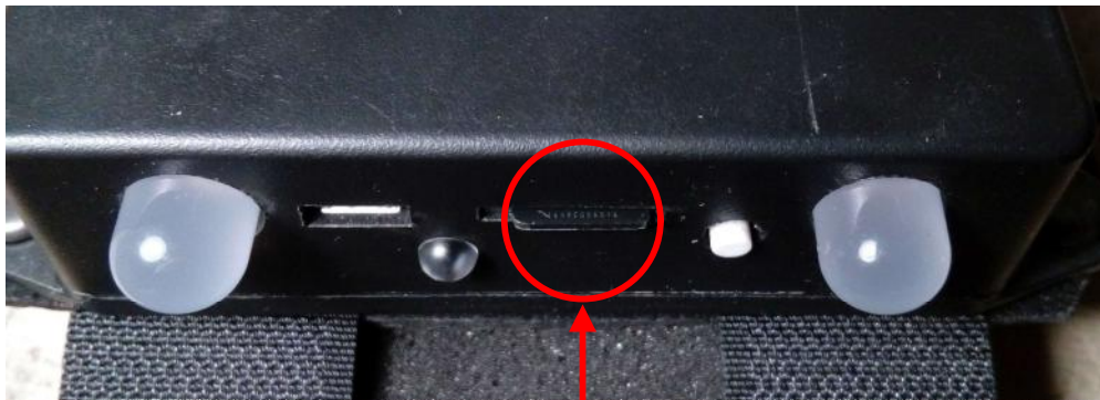
Micro SD card, in place (note that it is nearly flush with the case)
